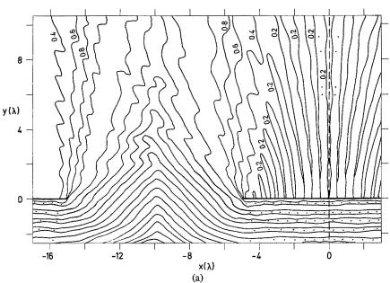
Figure 3-Solution for a double slit. (a) Lines of constant amplitude. Unlabeled lines have unit amplitude. Points of zero amplitude are shown by a dot; (b, facing page) Lines of constant phase. (c, facing page) Lines of energy flow. The axis of symmetry is represented by the dashed line.
