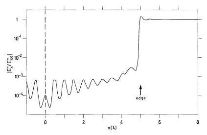
Figure 4-Tangential field  $E''_x$  in the plane of the slits (shadow side).  $E''_{x0}$  is the value of  $E''_x$  in the center of the slit aperture.
