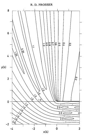
Figure 1-Solution for the semi-infinite plane: (a, above) lines of constant amplitude; (b, facing page) lines of constant phase (-----) and lines of energy flow (-----).
